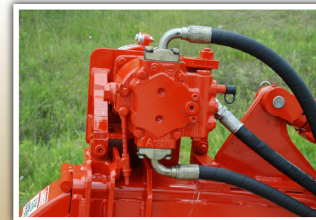
HYDROSTATIC DRIVE 3.3ci hydrostatic motor with 8cc functions gear pump, 16cc track drive gear pump and 5.4ci hydrostatic transmission
