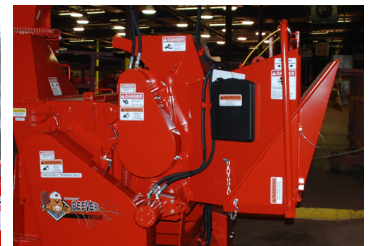
Folding Infeed Tray The folding infeed tray shortens transport lengths and increases maneuverability.
